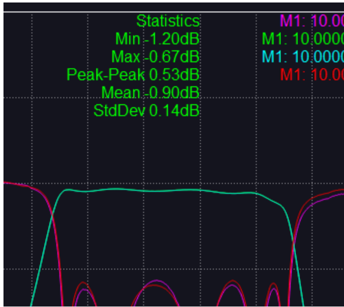
Figure 19 Example statistics measuring flatness of a passband filter.
